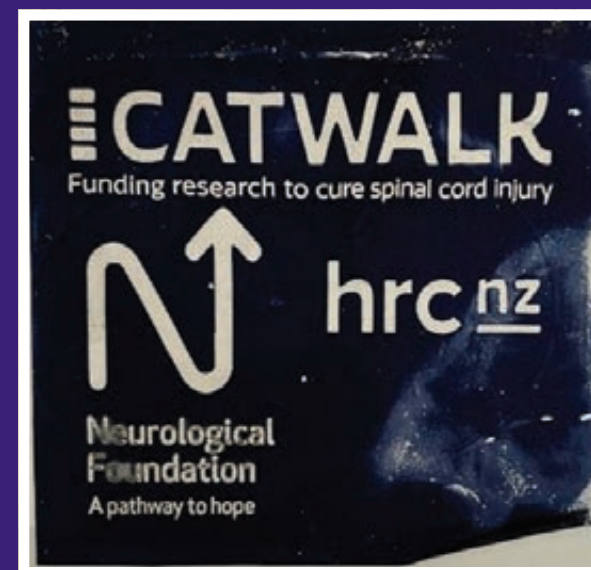
Figure 1: Stretchable and conductive material that we can pattern into a microelectrode array. In this image we are demonstrating the ability to pattern shapes by showing the CatWalk logo.
